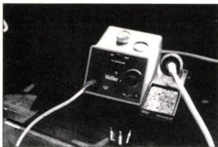
Fig. 2: A temperature controlled soldering iron station (in this case a Weller type), with the associated stand and essential sponge (see text for comments on techniques).
