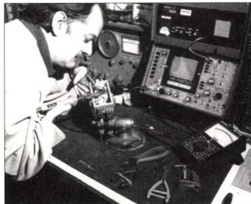
Ben Nock G4BXD hard at work on his workbench. The 'third hand' being provided by the portable vice on the bench. Note the rubber bands on the hand-tools, to provide necessary grip (see text).
