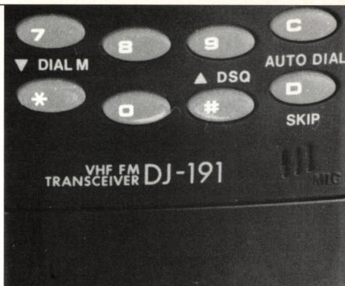
Unusually, the transceiver's microphone is mounted at the bottom of the front panel.
