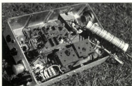
Fig. 4: A completed 3.5MHz c.w. transceiver built into a (recycled!) former television camera case! (see text).
